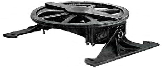
Webbed construction of the 18-24-30 Fifth Wheel for lightness without sacrificing strength
