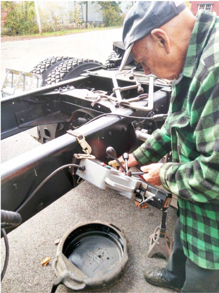
above left Jim Hall drills the frame for the step below left Jim Gordon masks before painting the roof
