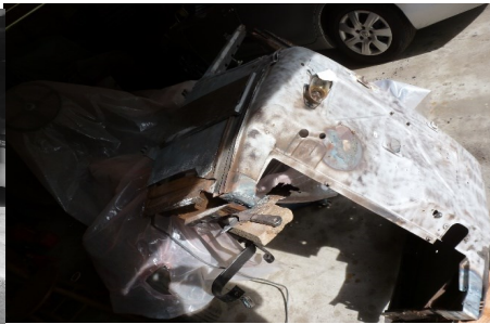
Cowl cleaned and ready for blasting.
