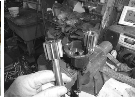
Pump gears show little wear, so reuse them.
