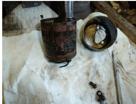
Clean oil pump screen and body
