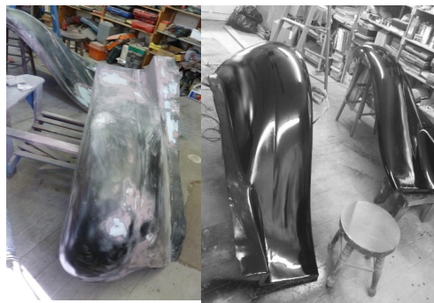
Fenders repaired and painted
