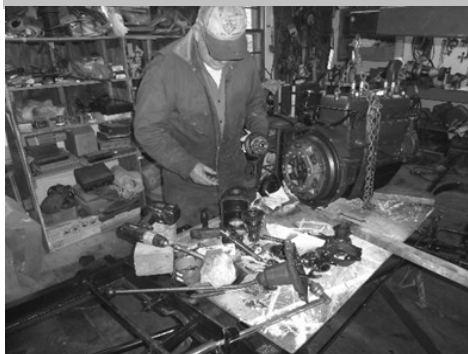
Inspect transmission parts
