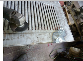
Weld repair to hood after sandblasting
