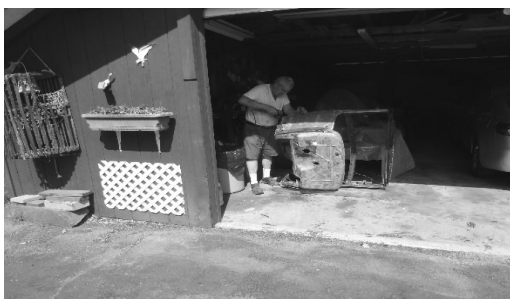
Grinding out patch of cowl
