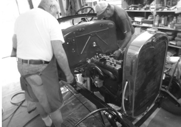
WITH THE COWL PRIMED AND PAINTED, YOU CAN ASSEMBLE THE COWL ONTO THE CHASSIS!
