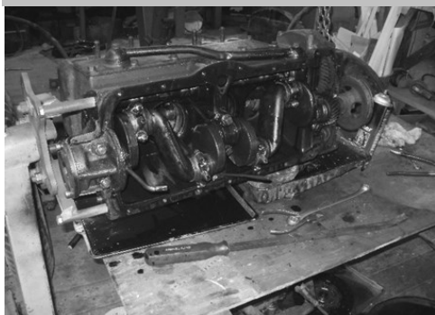
Engine, lower end ready to check
